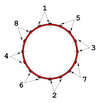
Final torque to be applied 35 lb.ft. (47 Nm)
