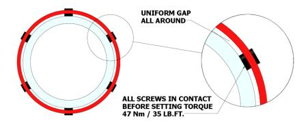
**Step 3.**Apply **35 LB.FT. (47 Nm)** according to the following patterns similar to wheel lug pattern tightening. Calibrated torque wrench is advised.
