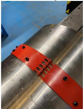
7. The installed stop collar can then be used to rest the centraliser during installation.
