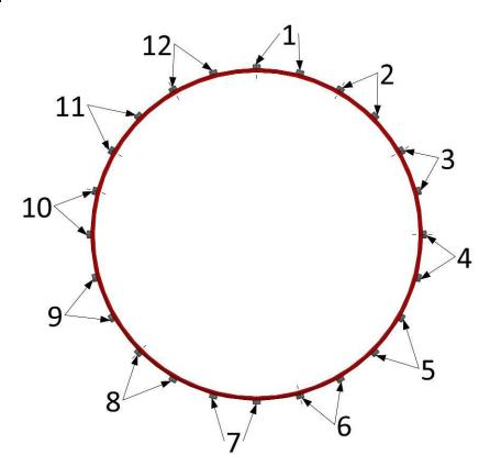
Final torque to be applied 35 lb.ft. (47 Nm)
