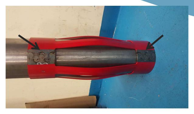
8. At this point the weld procedure can be followed in order to weld the centraliser interlocks together.
