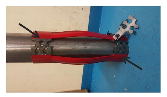
6. The interlock spacer can now be removed and disposed of by cutting the cable tie.
