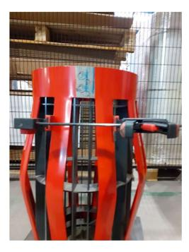
8. If the interlock gap exceeds 1mm when fitted to the pipe (pre-weld), then use a clamp on the bows to gently pull the interlock gap together.
