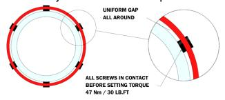
Apply torque @ 30 lb.ft. (40.7Nm)
