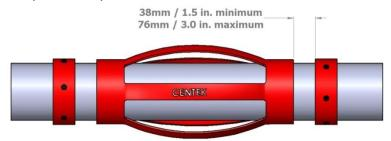
Set screw depth to be adjusted so collar is equal distant from casing on all sides.
