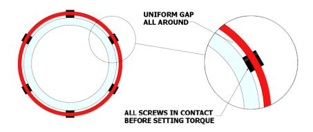
**Step 3.** Apply **20 LB.FT. (27 Nm)** according to the following patterns similar to wheel lug pattern tightening. Calibrated torque wrench is advised.
