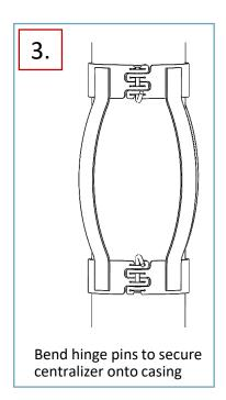
IMPORTANT! Centek do not recommend installation over stop collars or casing collars and doing so could affect the stated performance of the product
