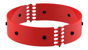
The 00SH provides a high-performance method of securing and protecting centralizers on the casing string. Made from the same material as our ultrahigh strength S2 Hinged centralizer, the 00SH utilizes a low profile, twisted hinge design for quick installation.
